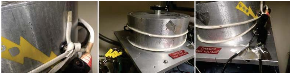
FIG. A.33. Heater Tape. (left) Tie one end of the heater tape to the handle of the ESD chamber. (center) Wrap the tape around the chamber. Make sure that the internal wire is not exposed and that the wire from the two separate tapes do not cross. (right) Tape the heater tapes to the ESD chamber using aluminum tape so that they do not move. This will stop them from falling across each other when they are hot. Only put aluminum tape over the part that does not heat up.
