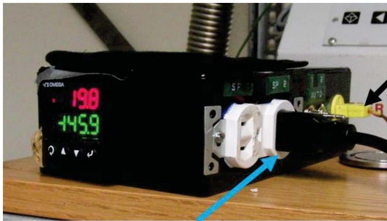
FIG. A.29. PID temperature controller box. The blue arrow indicates the power cord from the LN2 valve controller. The black arrow indicates where the ESD cryogenic reservoir TC cable plugs into the PID control box. The red value on the PID control box is the temperature ( ^{\circ}\text{C} ) read from the TC cable plugged into it. The green value is the target temperature ( ^{\circ}\text{C} ). For more information on the PID box, read its separate documentation.
