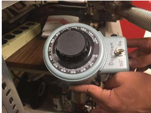
FIG. A.34. Transformer. Variac transformer setting corresponding to an outer temperature of approximately 100 °C and an inner temperature of ~82 °C.
