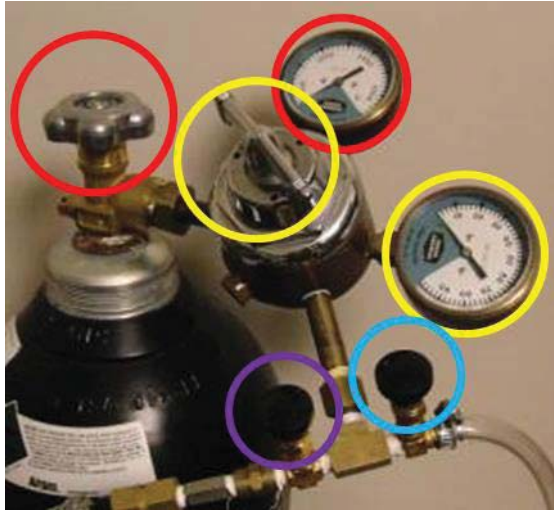
FIG. A.25. N 2 gas tank next to glove box. The tank is controlled by the valve circled in red. Turn it CCW until the gauge circled in red jumps, this gauge indicates the remaining pressure in the tank. The valve in yellow controls the pressure coming out of the tank, which is read by the gauge, circled in yellow. The blue valve directs gas to the ESD and bakeout chambers, while the purple valve directs gas to the glove box.
