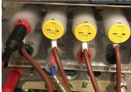
FIG. A.30. TC connections on switch box. Left to right, cryogenic reservoir, A side, and B side TCs.
