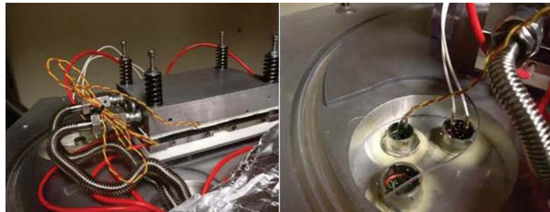
FIG. A.31. Internal temperature measurements. TC inserted into the cryogenic reservoir (left). TC feedthrough connections (right).
