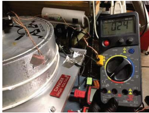
FIG. A.32. External temperature measurements—Aluminum tape is used to attach the TC to the chamber and is read with the multimeter.
