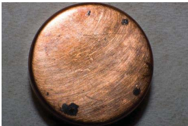
FIG. A.35. Black carbon char marks left on an electrode from a large ESD event through a polymer.
