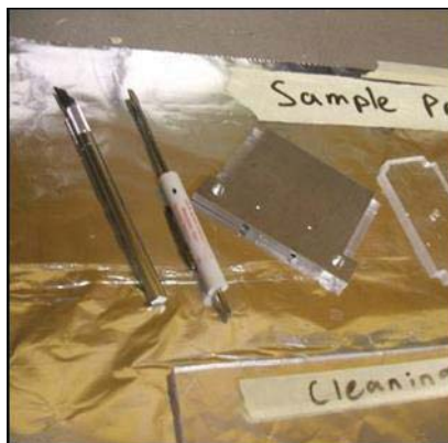
FIG. A.2. Materials needed for sample prep: (left to right) knife, screwdriver, HV plate, and sample template.
