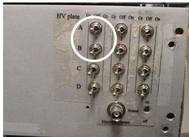
FIG. A.22. Sample plate switches outlined in white. “A” switch corresponds to sample plate A and the “B” switch likewise corresponds to sample plate B. Only one switch should be in the on position during a run and it should only either be the “A” or the “B” switch.
